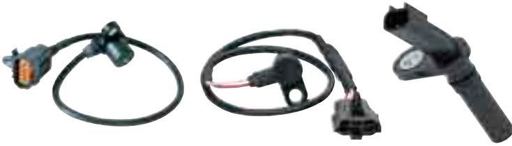
**Inductive Sensors** use electromagnetic induction principles to generate an output voltage indicating crankshaft/camshaft speed and position. The sensor consists of a coil winding wrapped around an iron core and is located near the sensing surface (e.g. crankshaft pulse ring, flywheel teeth).
