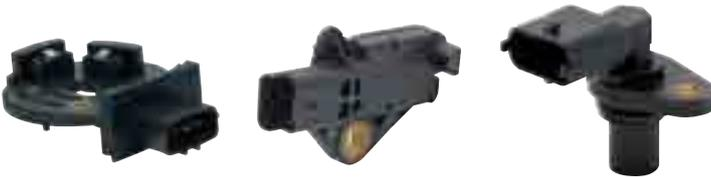
**Hall Effect Sensors** use Hall Effect principles to generate an output voltage indicating crankshaft/camshaft speed and position. The sensor consists of a permanent magnet and semi conductor incorporated into an integrated circuit (Hall I.C.), along with a steel vane driven by the crankshaft/camshaft.
